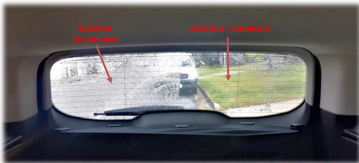
Image 1 – LAMINATE is SAFE: View is not blocked for laminated one way vision when it rains
