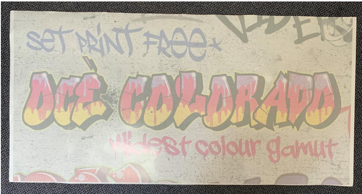
Photo 4: Sample graphic removed, leaving Universal Liner. Every perforation of the art area has ink. Not one single hole had ink bridging.
