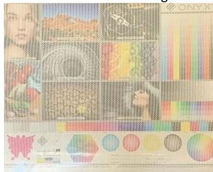
Photo 2: Face film removed, ink on liner in locations where the holes were. No ink bridged.
