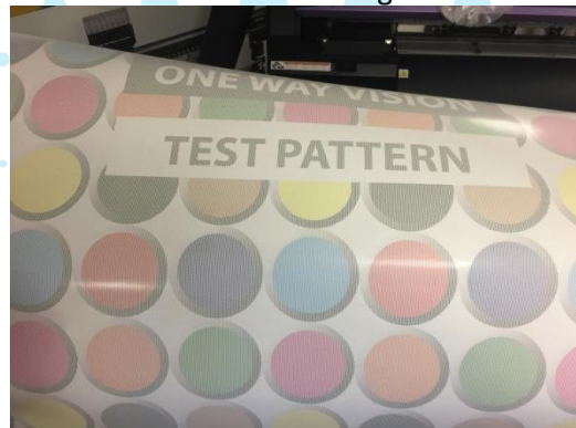
Image 2: Face film removed, ink on liner in locations where the holes were. No ink bridged.
